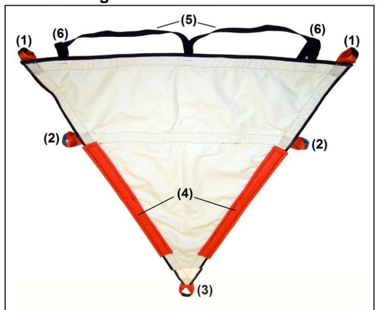
The rescue cloth is used for raising and abseiling people (rescuing from heights and depths) in a sitting position. Put the rescue cloth on the back of the person to be rescued, pull the 2 connecting loops (1) forwards by placing them under the armpits, pull the middle connecting loop (3) with the preassembled tape sling between the legs upwards.
